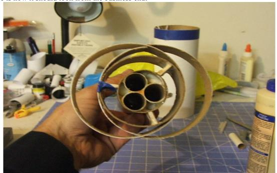
9. Next, the fins are glued onto the BT60 lined up with the tail ring stand offs.
