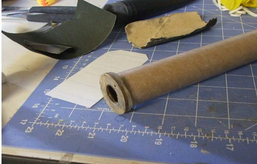
4. The 3 motor mount tubes are then glued together and dry fitted into the BT60 to hold the tubes together for the glue to fully dry. After the glue has dried the assembly is glued into the BT60 flush with the end of the tube. I then tore some paper from the shipping box and crumpled into small balls. Soaked with white glue these balls are then used to fill the gaps around the motor tubes.
