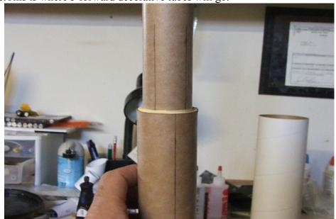
6. The tail ring is rebuilt using 5 minute epoxy. 2 1" lengths of the BT101 tube are cut. 5 2" long tubes were cut from the BT5 tubes. The fronts of the BT5's were cut at a 45 degree angle..
