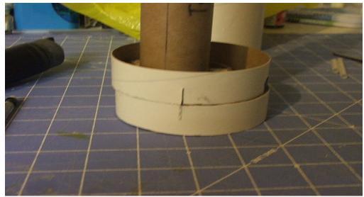
8. The BT101 tubes are now interlocked and glued to the tail ring tube.
