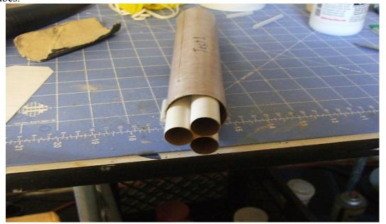
5. Next, the BT55 with the glued on centering ring is inserted into the BT60 until the centering ring is butted up to the front of the motor tubes. Then, the BT55-BT60 centering ring is slid down and glued flush to the end of the BT60 tube. Using 'Template Widget' a fin marking guide for BT55 with 5 fins is printed out and the tube is marked. The lines are extended for 3" along the tube. This is where 5 forward decorative tubes will go.
