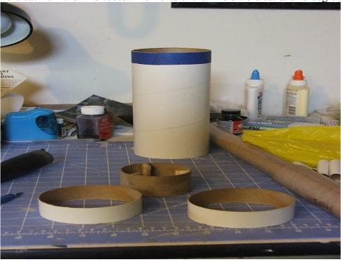
7. The tail ring is then glued to the base of the BT60.Next the 2 BT101 rings are stacked with one side on opposing sides of the tail ring tube. The cross pints of the BT101 tubes are marked and 1/2" long slits are cut so the rings can 'interlock'.
