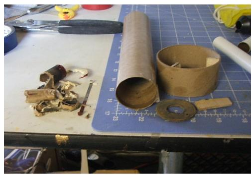
2: New motor mount tubes were then cut from the BT20 tube. This will be a 3x18mm cluster rocket. After the tubes were cut engine blocks were glued into the forward end of the tubes.
