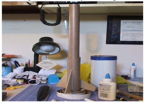
10. The 5 forward decorative tubes are now glued to the BT55 tube with the aft end of the tubes butting up to the BT60 tube.
