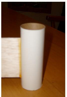
Next, glue the balsa fins along the other four lines, also even with the bottom of the BT-70 body tube. Use super glue to attach the fins, then wood glue to fillet.
