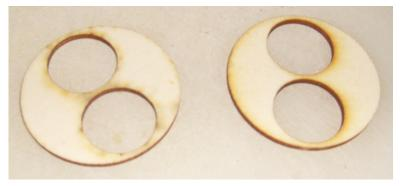
Test fit and sand the centering rings if necessary. Use wood glue to glue one centering ring flush with the top of each tube and the other even with the 1/2" marks on the tubes.
