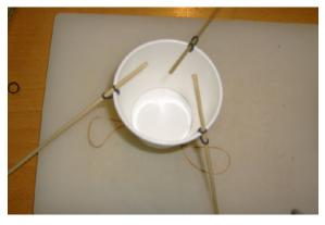
Next, slide a skewer through both loops of one black rubber band, then do the same with the other two. Slide the other end of each skewer through the corresponding brown rubber band, then loop each rubber band again to tighten the bands.
